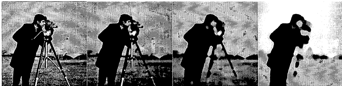
Figure 4. Selected levels of a locally monotonic scale-space derived from the original cameraman image of Figure 5. From left, original 256-graylevel image (256 x 256 pixels), scale-space levels corresponding to structuring element diameters of 3, 7, and 11 pixels.
