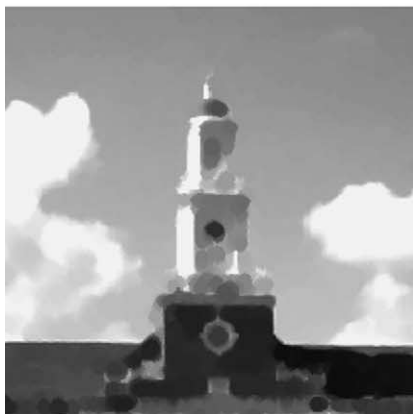
Fig. 10. Close scale-space derived from Fig. 6 using structuring elements of radius 1, 2, and 4 pixels (from top).
