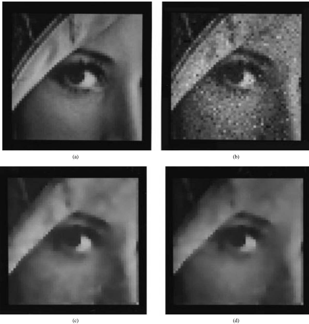
Fig. 3. (a) Original “eye” image; (b) corrupted image (Laplacian noise, SNR = 9 dB) used as input for results in (c) and (d); (c) after two iterations of anisotropic diffusion with DC 2 ( k = 25 ); (d) After one iteration of multigrid anisotropic diffusion with DC 2 ( k = 25 ).
