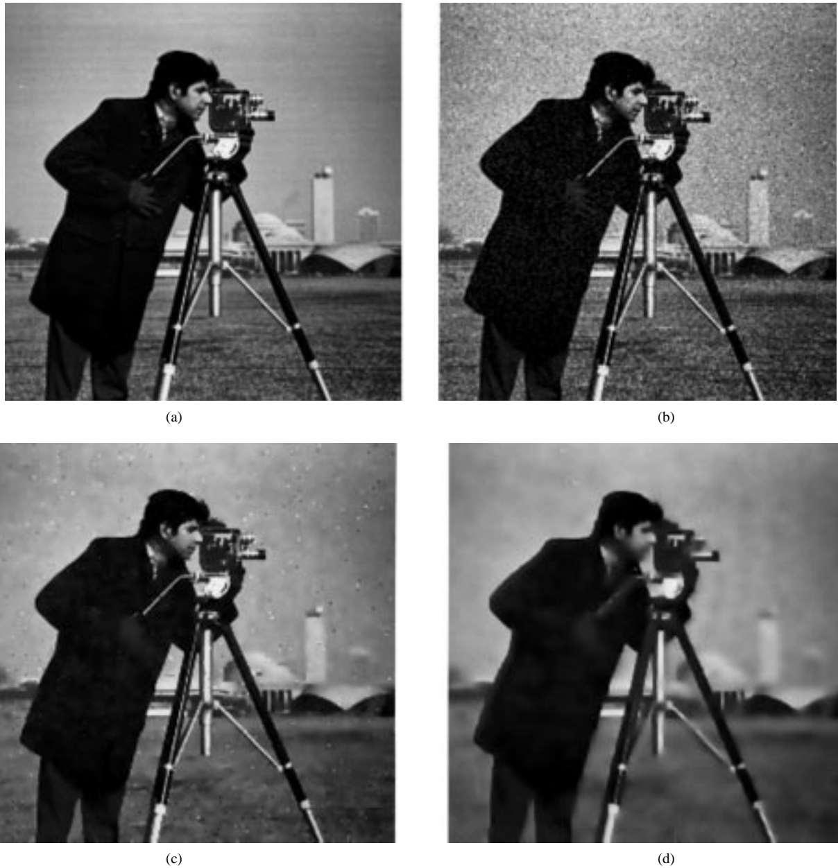
Fig. 4. (a) Original cameraman image; (b) corrupted image (Laplacian noise, SNR = 13 dB) used as input for results in (c)–(f) and Fig. 5(a) and (b); (c) after eight iterations of anisotropic diffusion with DC 1 ( k = 25 ); (d) after eight iterations of anisotropic diffusion with DC 2 ( k = 25 ).
